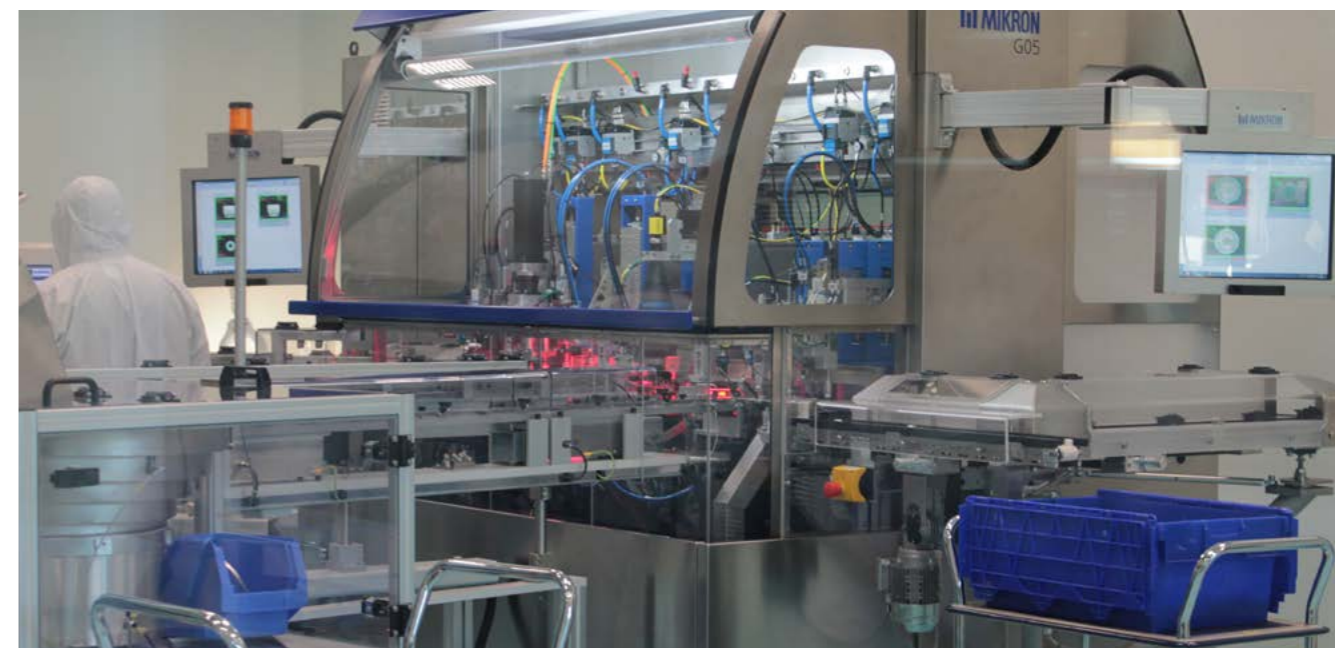
Automated assembly equipment for RayDyLyO
