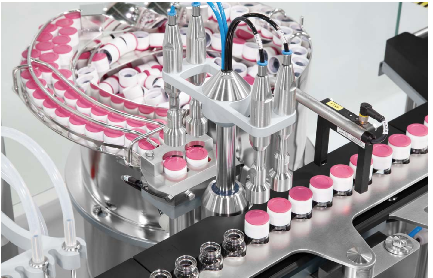
The pick & place station handles RayDyLy o caps by vacuum.
